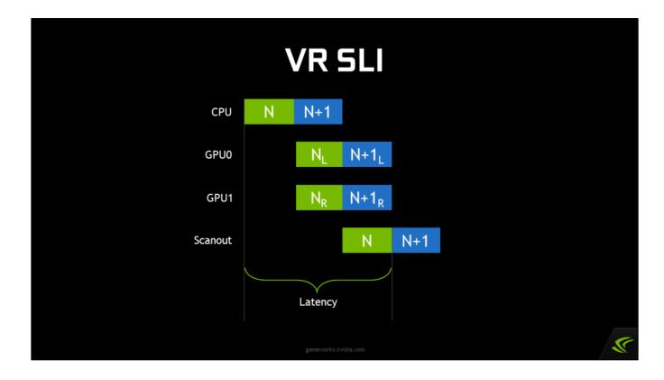
A better way to use two GPUs for VR rendering is to split the work of drawing a single frame across them — namely by rendering each eye on one GPU. This has the nice property that it improves both framerate *and* latency relative to a single-GPU system.
