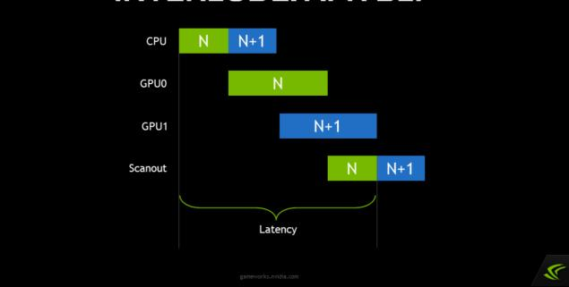
Before we dig into VR SLI, as a quick interlude, let me first explain how ordinary SLI normally works. For years, we've had alternate-frame rendering, or AFR SLI, in which the GPUs trade off whole frames. In the case of two GPUs, one renders the even frames and the other the odd frames. The GPU start times are staggered half a frame apart to try to maintain regular frame delivery to the display.
