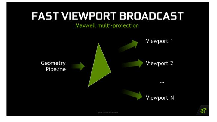
The key thing that makes this technique a performance win is the multi-projection hardware we have on NVIDIA's Maxwell architecture – in other words, the GeForce GTX 900 series and Titan X.
