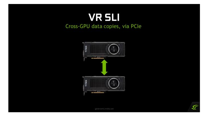
And of course we need to be able to transfer data between GPUs. For instance, after we've rendering both halves of the stereo pair, we have to get them back onto a single GPU to output to the display. So we have an API call that copies a texture or a buffer between two specified GPUs, using the PCI Express bus.
