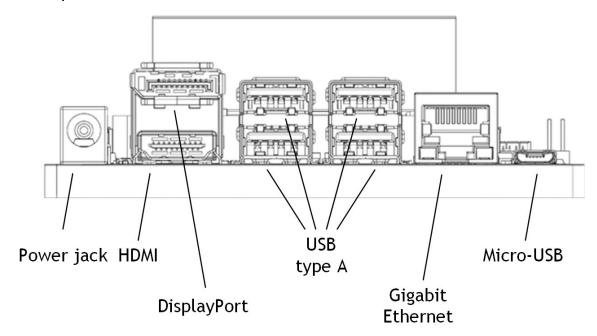
Developer kit module and carrier board: rear view
