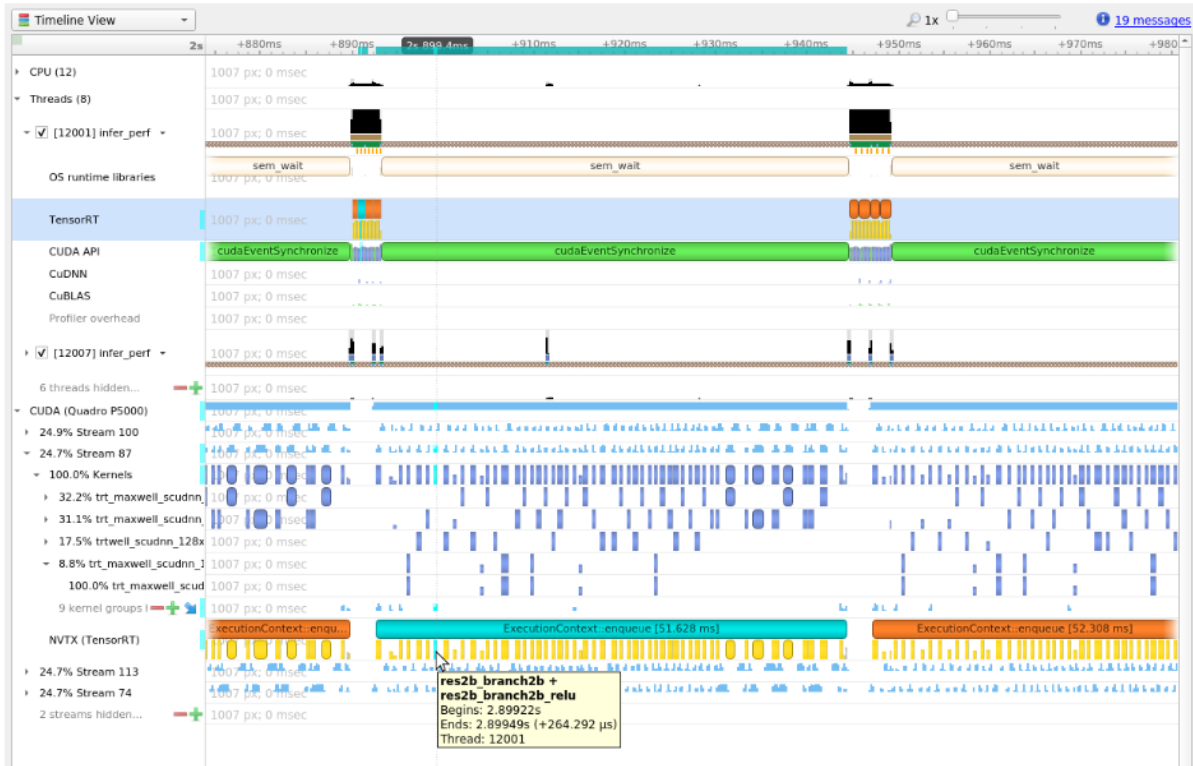
Figure 17. The kernels actually run on the GPU, in other words, it shows the correlation between the layer execution and kernel launch on the CPU side and their execution on the GPU side.
