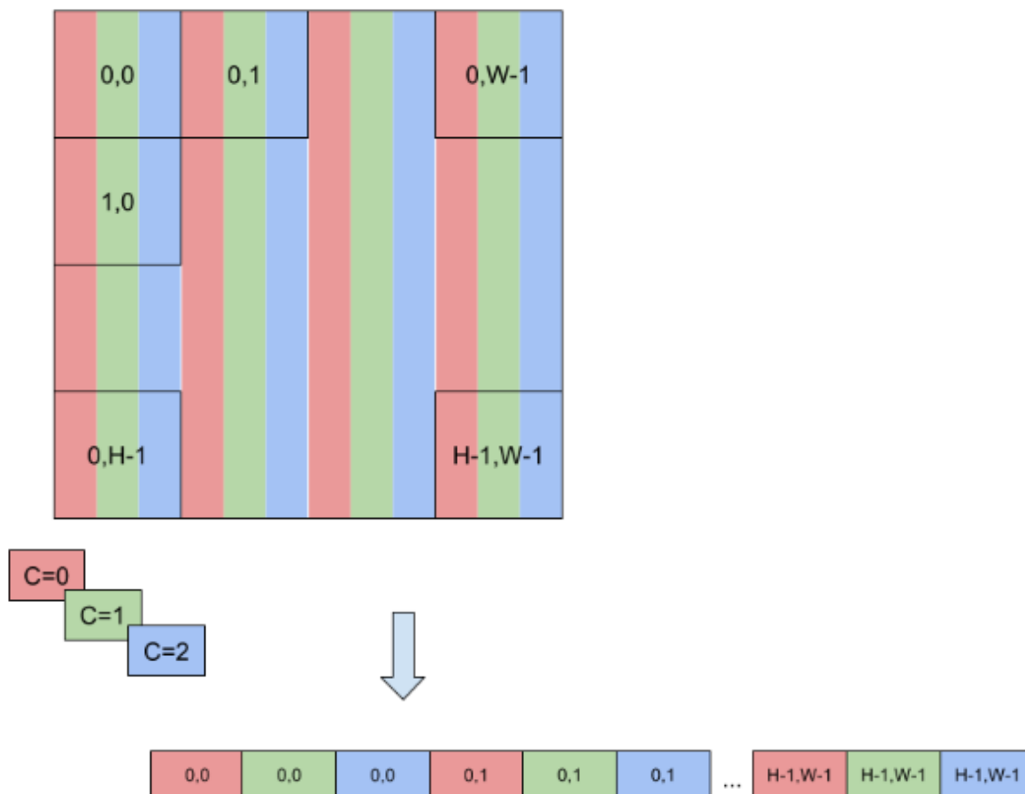
Figure 18. Layout format for HWC: The image is stored as a single H \times W matrix, whose value is actually C-tuple, with a value per channel; all the values of a point (pixel) are stored contiguously.
