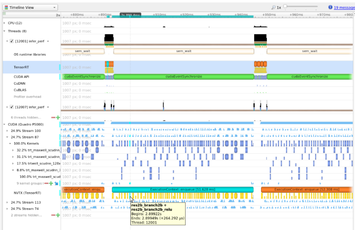
Figure 18. The Kernels Run on the GPU
