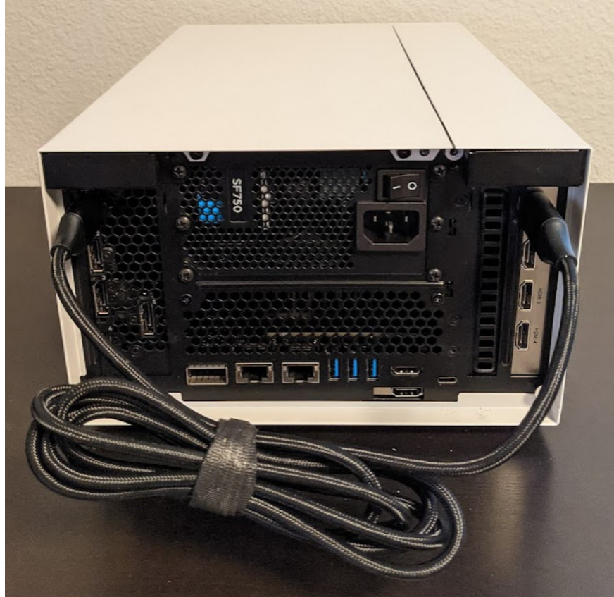
Fig. 30.2: DP-to-HDMI Cable Between GPU and AJA KONA HDMI Capture Card (Channel 1)
