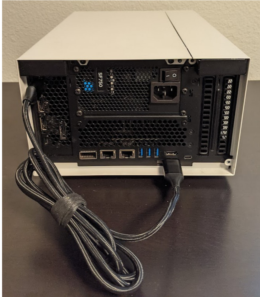
Fig. 30.1: DP-to-HDMI Cable Between GPU and Onboard HDMI Capture Card
