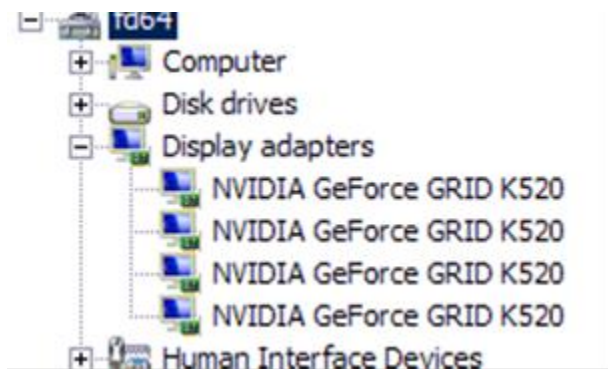
Figure 1. Example System with Two GRID K520 Boards Showing Four GPUs
